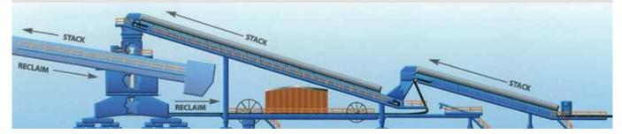
**Scissors-Type Tripper** is also used when material enters and leaves the storage area from the same end of the yard. This tripper utilizes a separate elevating conveyor to direct the material to the centerline of rotation for stacking.
