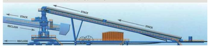
**Articulating Tripper** is used when material enters and leaves the storage area from the same end of the yard. By articulating the tripper structure, this section can be lowered (retracted) for reclaiming operation.
