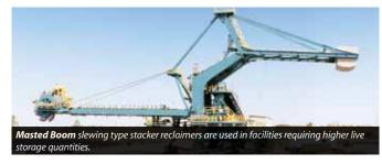
**Masted Boom Configuration** is designed for use in applications where extended boom length over 125 feet (38 meters) is necessary. The added support reduces excessive boom flex inherent in long-reaching stacker reclaimers or where high digging forces cause unacceptable boom tip deflection.
