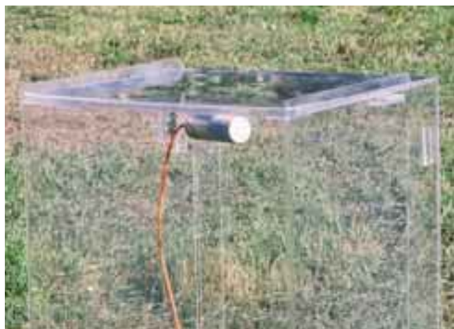
In soil respiration measurements on the ground surface, the CO 2 efflux is measured inside a box that is placed on the ground at the site under examination.
