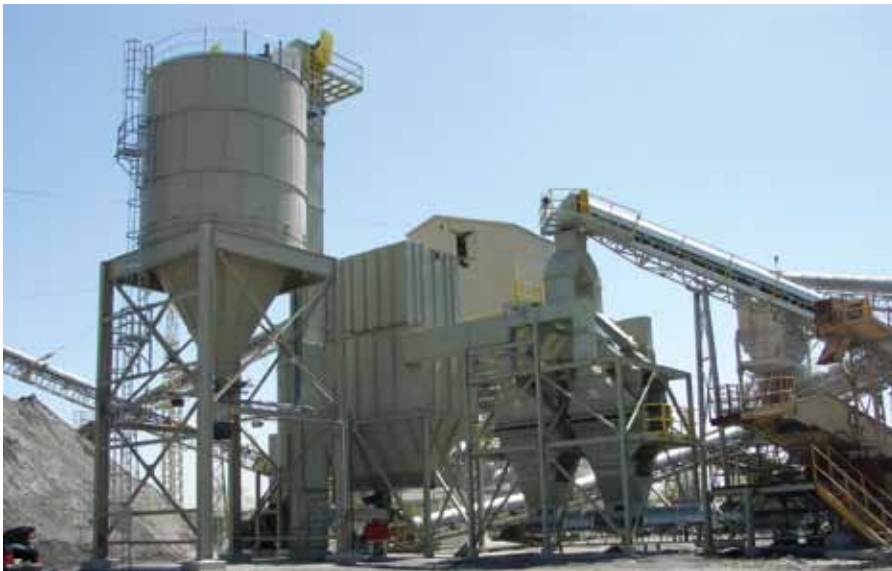
Dry classifying uses no water, providing a very environmentally friendly and economical classifying solution. Metso air classifiers provide a full system solution with an alternative to wet classifying.
