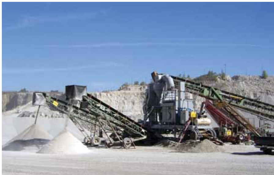
Centrifugal unit in series with gravitational inertial unit. 75 tph mobile unit, transportable to job sites, incorporates quick set up hydraulics and ceramic liners for wear protection.
