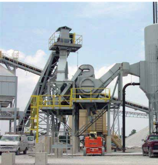
Centrifugal unit in series with gravitational inertial unit. 75 tph mobile unit, transportable to job sites, incorporates quick set up hydraulics and ceramic liners for wear protection.
