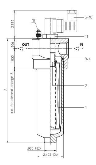
1) Connect the stand grounding tab to a suitable earth ground point.
