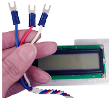
Figure E.11—Switch wires showing two-prong connectors
