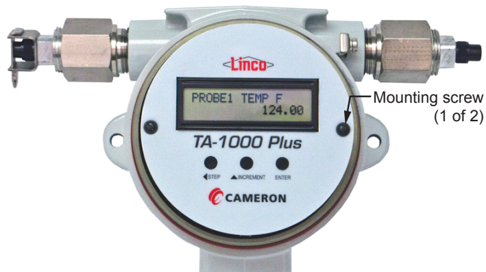
Figure 5.13—Faceplate showing location of mounting screws
