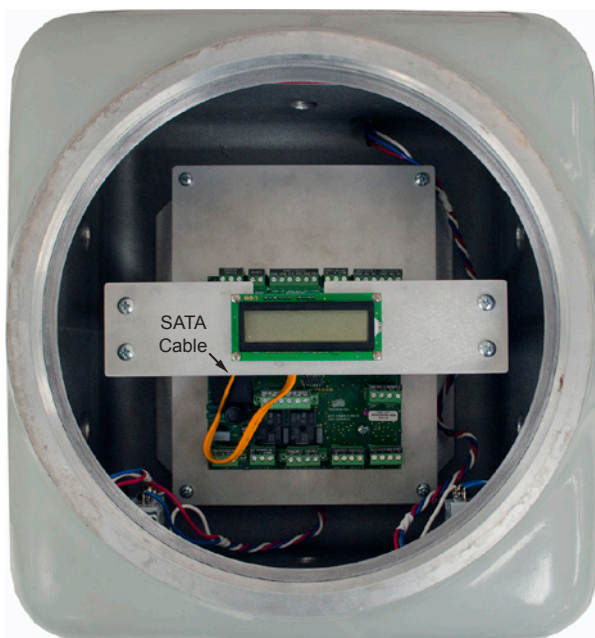
Figure E.15—New display and mounting bracket showing SATA cable location for reference
