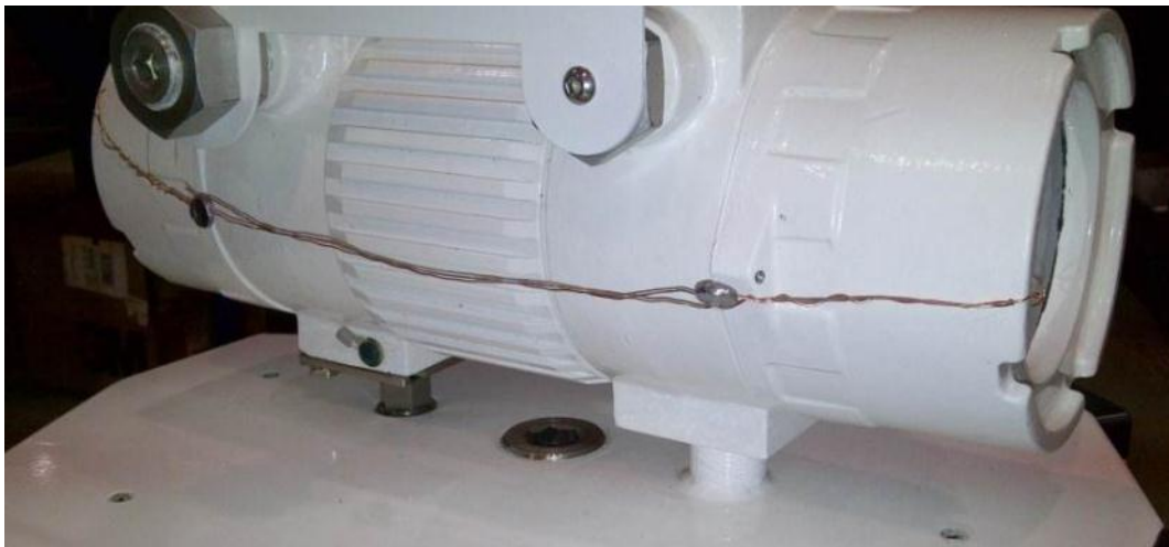
Figure 10-3: Depiction of Seal Wire on Transmitter Enclosure
