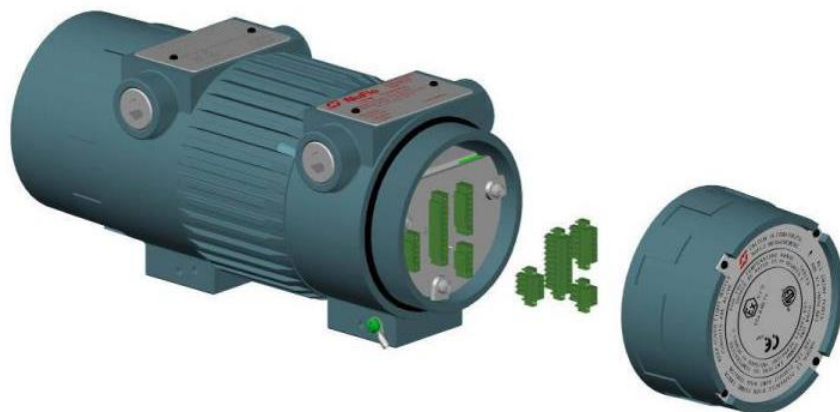
Figure 4.2: Transmitter with Rear Cover Removed (Communications Option 1 Backplane Shown)
