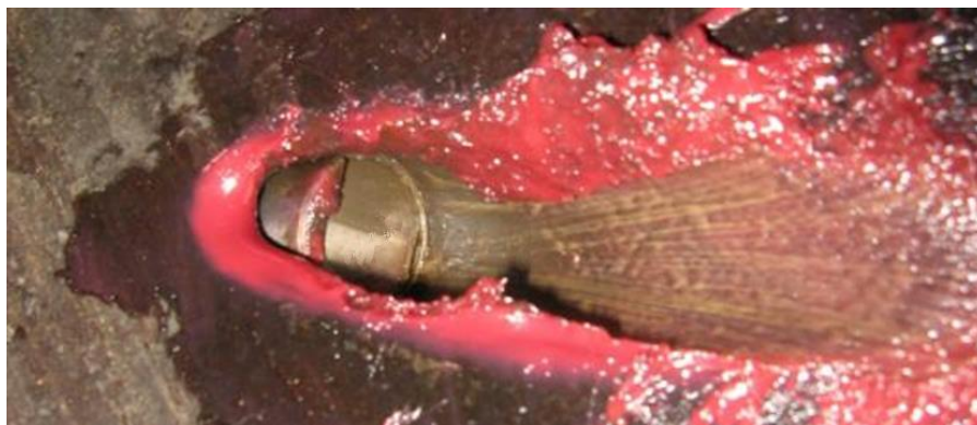
Figure 7.1: Result of purging transducer housing and cavity
