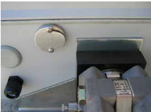
Figure 3.22—Console serial port connector shown with the cover in place at the bottom of the Scanner 1141 enclosure (left) and shown with the cover unlatched (right)
