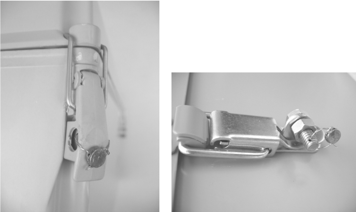
Figure 2.3—Seal wire installation on an 1141C latch (left) and an 1141L latch (right)
