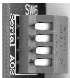
Figure 3.27—Auxiliary serial port switch with all RS-485 connections enabled
