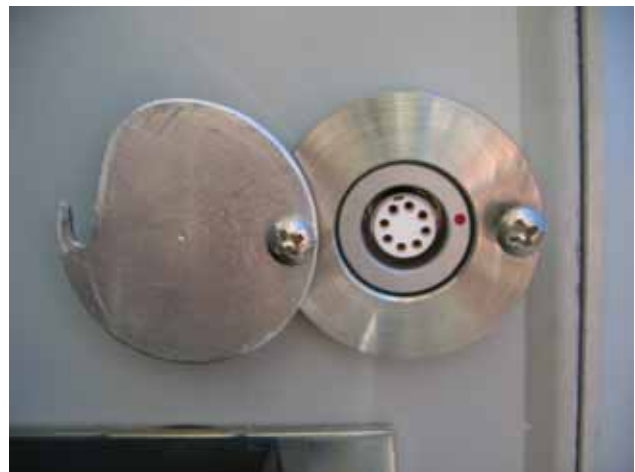
Figure 3.22—Console serial port connector shown with the cover in place at the bottom of the Scanner 1141 enclosure (left) and shown with the cover unlatched (right)
