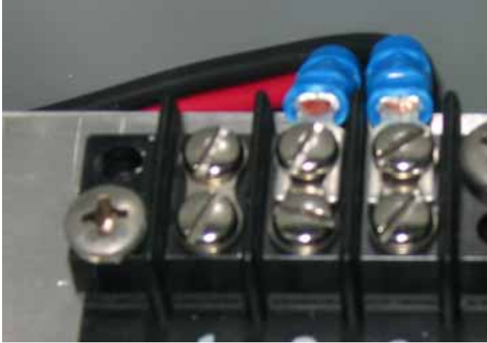
Figure 2.10—Barrier terminal block for wiring a solar panel or power supply to the Scanner 1141
