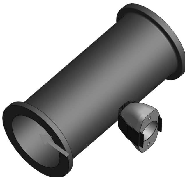
Figure 12. Installing the sleeve to the pusher.
