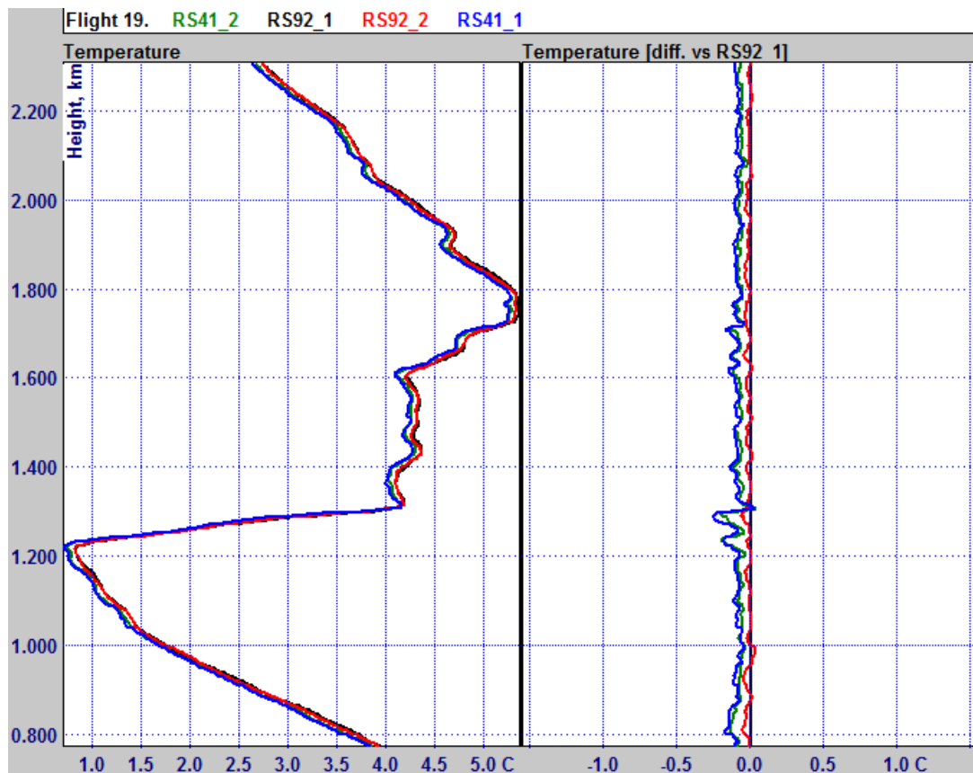
Figure 13 – Example from flight 19 showing the measured temperature differences of the RS41 radiosondes and RS92_2 radiosondes relative to the RS92_1.
