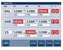
A customer-specific controller's display was designed for the FAA Runway Visual Range System using Vaisala AviMet°'s new display development tools.
