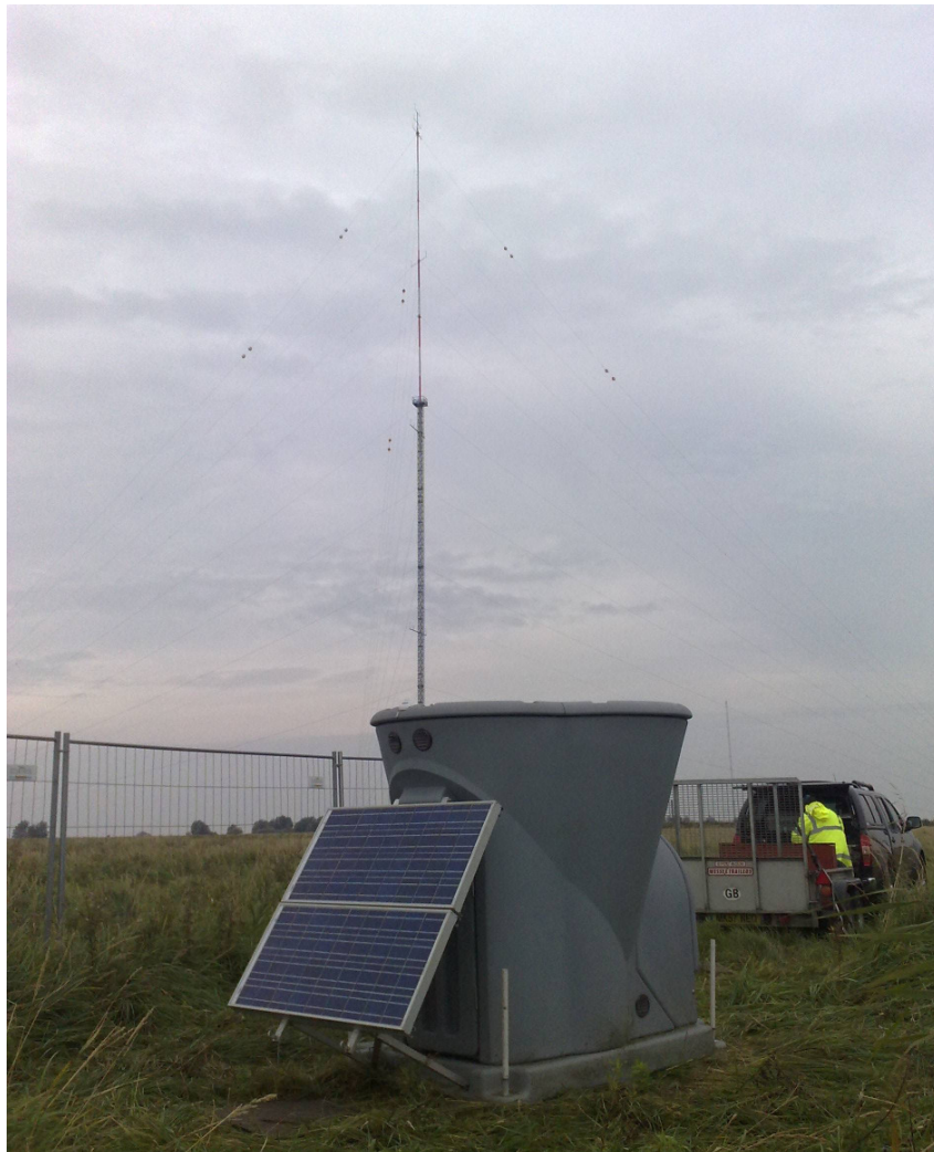
Figure 4: The Triton under test installed close to the met tower near Rysum.
