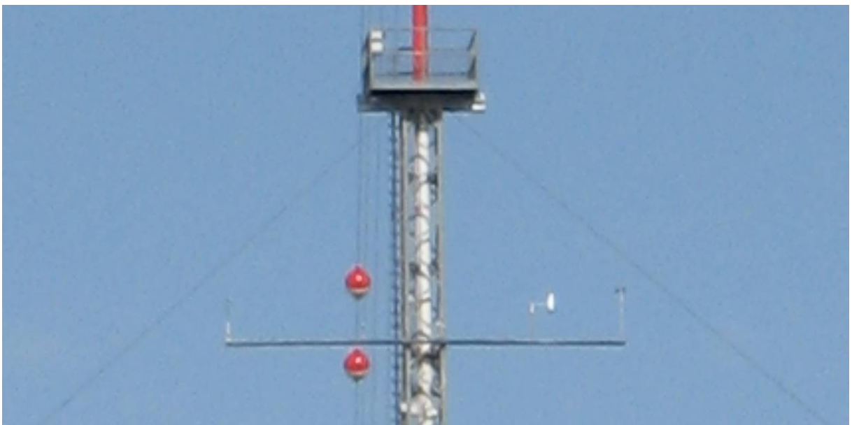
Figure 65: Photo of the sensors and booms at a height of about 72 m above ground
