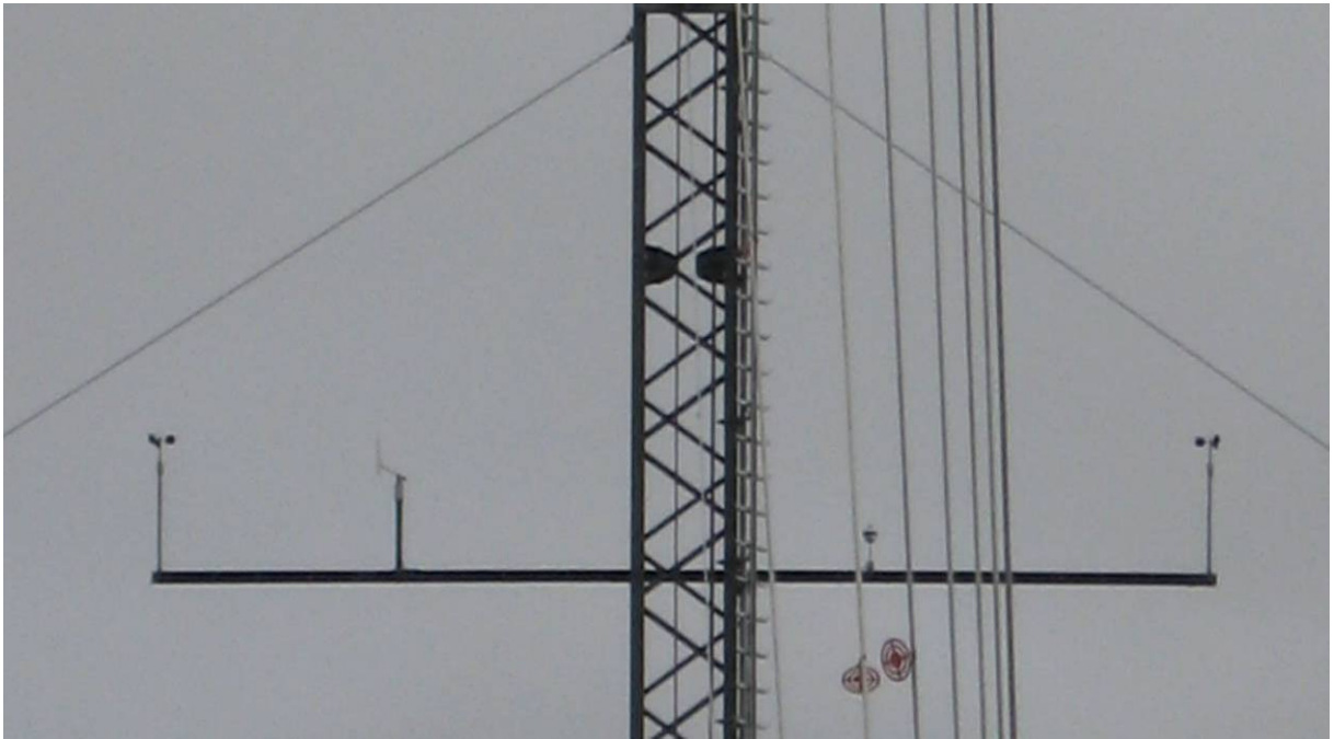
Figure 66: Photo of the sensors and booms at a height of about 35 m above ground
