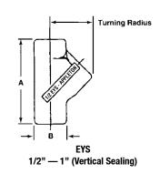
\* Per NEC 501.15(C)(6), seals in Class I, Division 1 and 2 must be limited to conductor fill of 25% of cross sectional area of a rigid metal conduit of the same trade size unless approved for higher percentage fill. See 40% fill sealing fittings. ① Turning radius with cover or plug removed.
