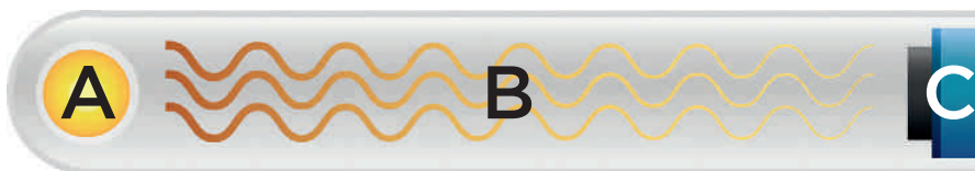
Figure 1. Infrared absorption of CO 2 molecules can be detected with an infrared detector. A: Infrared source. B: Optical path. C: Detector.
