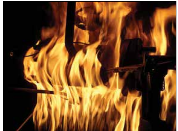
During fire testing to API 607 6th Ed.
