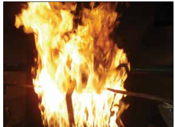
During fire testing to API 607 6th Ed.
