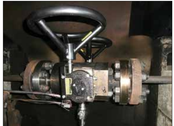
Compact, double block-and-bleed design (prior to fire testing)
