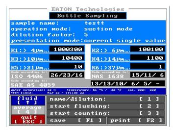
After the completion, the measurement can be saved by using [ F1 ], print by using [ F2 ],
