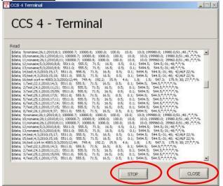
NOTICE If an empty terminal window appears, the correct COMport has to be selected. After changing the COM-port the terminal connection has to be checked again.
