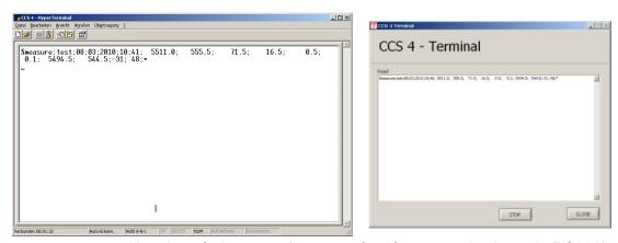
Notation of "data transfer – transfer of measured values via RS232" selection of "reading by CCS 4 data manager".
