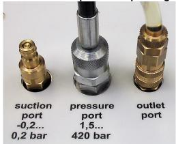
Connections from the left to the right: suction port, pressure port and outlet port for the return line.
