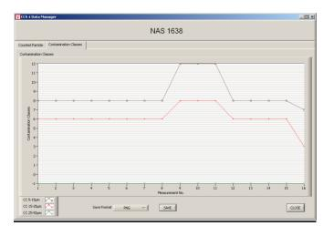
Diagram of the contamination class according NAS 1638.
