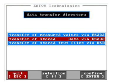
With the [↓↑] – keys switch to the menu for data transfer of the saved values by using the RS232-interface and confirm with [ENTER].
