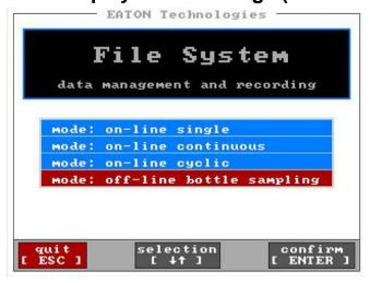
Select the "off-line bottle sampling" by using the [↑↓] – keys and confirm with [ENTER].
