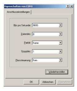
• Set up the transfer conditions at the computer as follows:
