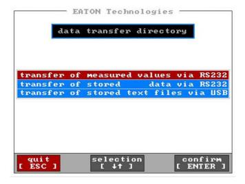
With the [↓↑] – keys switch to the menu "transfer of measured values via RS232" and confirm with [ENTER].
