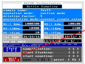
NOTICE If the measurement is saved with [F1], this measurement can't be use for the averaging.
