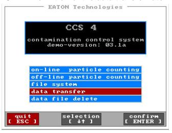
In the main menu of the CCS 4 select the menu "data transfer" by using the  $\lceil \uparrow \downarrow \rceil$  – keys and confirm with [ENTER].
