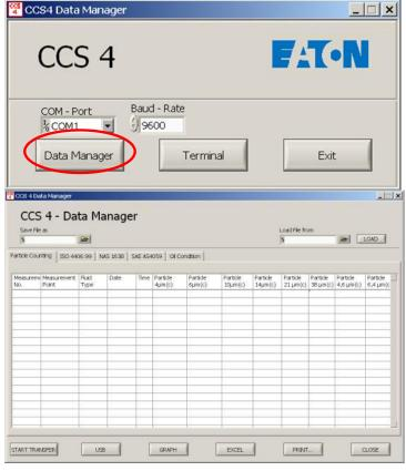
Clicking the button "Data Manager" allows the data transfer and the processing of the transmitted values.
