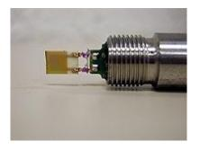
In addition, a temperature sensor is installed for precise temperature measurement of the fluid during the measurement.
