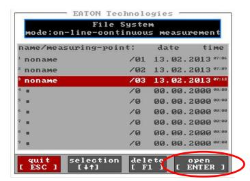
Select the saved measurement with [↑↓] and open the data set with [ENTER].
