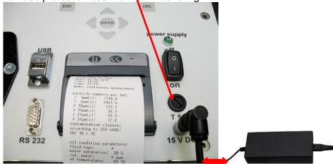
Switch on the CCS 4 with the "power supply" – switch to ON. (visible by the green control diode)
