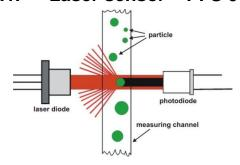
The laser sensor operates based on the light-blockade principle and generates an output signal depending on the particles' sizes. This is received, processes and classified by corresponding electronics.
