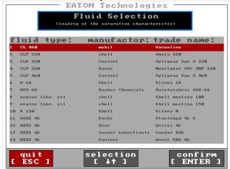
Select the fluid using the  $[\downarrow\uparrow]$  – keys (selection is highlighted red) and confirm with [ENTER].
