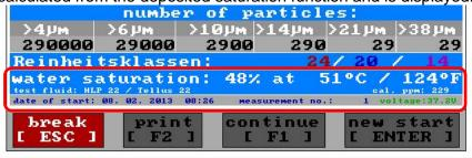
The relation to the detected saturation values and the data, after Karl Fischer method accounted ppm (mg/kg), is calculated then evaluated by the detected and deposited 100% saturation curve (100% saturation = f(T)) and the simultaneously measured fluid temperature and is indicated at the display.
