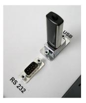
• Load the main menu and then insert the USB – stick in the USB-connection port of the CCS 4.
