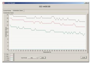
Display of the contamination classes according to ISO 4406:99.
