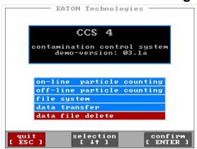
Select in the main menu of the CCS 4 the menu "data file delete" by using the [↑↓] – keys and confirm with [ENTER].
