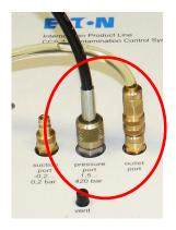
• In the **pressure operating mode** the provided high pressure hose (minimess hose) is being connected with the CCS 4 - **[PRESSURE PORT]** and the hydraulic system.
