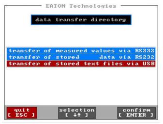
With the [↓↑] – keys switch to the menu for transferring of the stored TXT-Files via USB.
