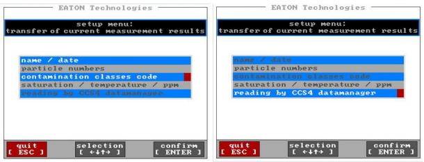
• Select with the  $[\downarrow\uparrow]$  – keys, which parameters are to be shown and activate with the  $[\leftarrow\rightarrow]$  – keys. (The selected parameter appears white.)
