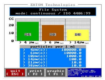
Display of the measuring data, the sample name, the date/ time, the temperature and the water saturation.
