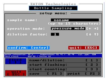
Enter the sample name, the dilution factor and the operating mode by using the [← →] and the [↓↑].
