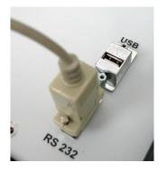
Connect the CCS 4 with the external computer using the RS232 – interface cable.
