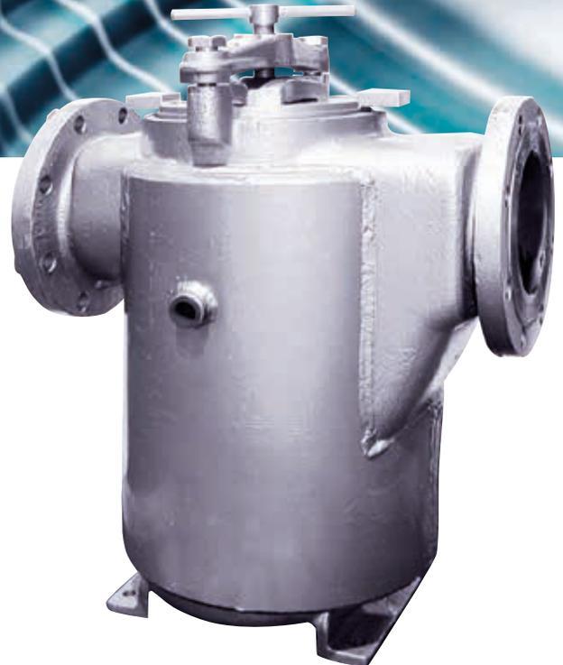
The Model 72SJ is for applications in which materials must be kept hot to remain fluid. Examples are chocolate, asphalt, resins and polymers. By circulating steam or a heat transfer fluid through the strainer jacket, the strainer body temperature remains constant.
