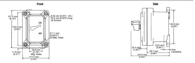
• For Class I, Division 1 applications sealing fittings must be field installed adjacent to enclosure on all conduit runs.
