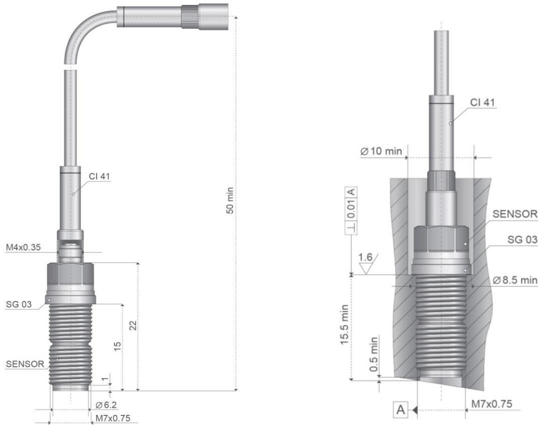
The sensor can be screwed directly into the object to be measured. The sensor rear side ( $\varnothing$  8.45 mm) seals the sensor in the mounting hole. Rapid changes in pressure are best detected when the volume in front of the membrane is kept as small as possible.
