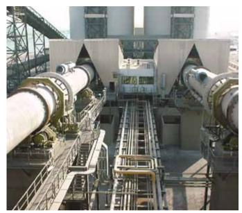
Two 250,000 MPTY Rotary kiln coke calciners
