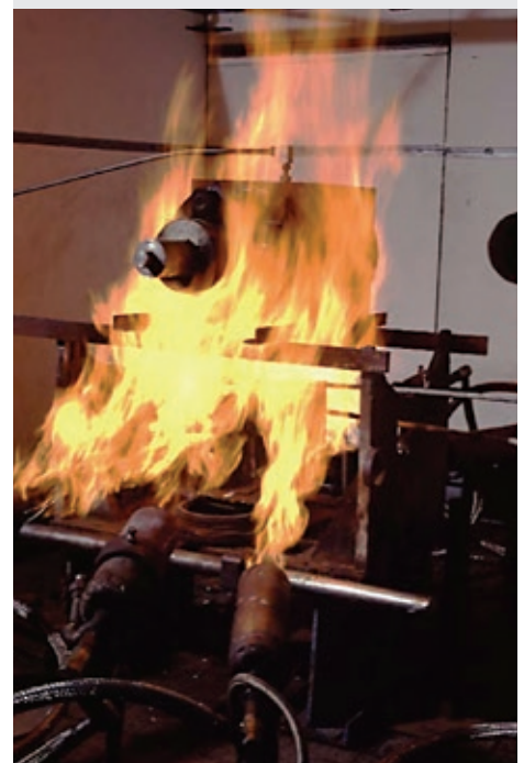
API 6FA choke fire testing
