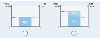
Effect of H<sub>2</sub>O and H<sub>2</sub>O<sub>2</sub> on relative saturation (RS) and relative humidity (RH)
