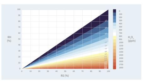
As an example, at 20 °C and 500 ppm hydrogen peroxide, the humidity level 25%RH is equivalent to 60%RS. When this gas mixture starts to condense (relative saturation being 100%), relative humidity is 45%.
