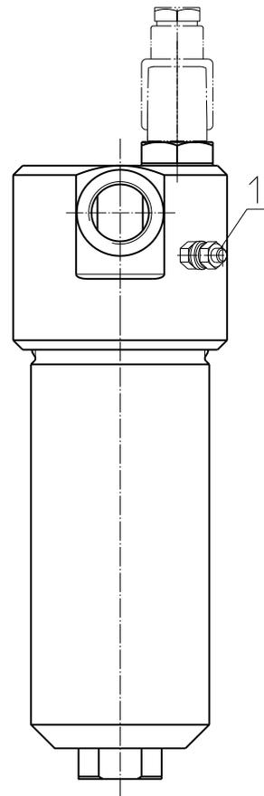
1) Connection for the potential equalization, only for application in the explosive area.
