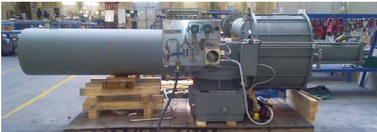
Cameron's LEDEEN® actuator mounted on a DYNATORQUE D-Stop partial-stroke test device.
