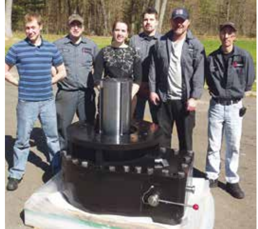
D-Stop devices are built for both large and small valves. This DT4000 D-Stop will fit between a large pneumatic actuator and a 36" 600# ball valve installed on an offshore platform.
