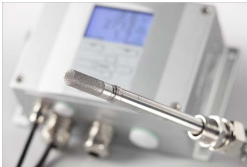
Installation of the DMT348 probe through a ball valve allows the user to remove the probe from a compressed air pipeline without the need to depressurize the system. The probe depth is adjustable.
