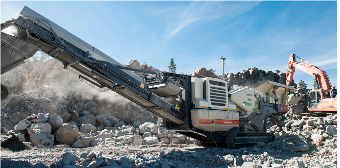
The Lokotrack® LT106™ mobile jaw plant operated by Pärhä Ltd. in Finland can be safely controlled from the cabin of an excavator using a wireless connection.
