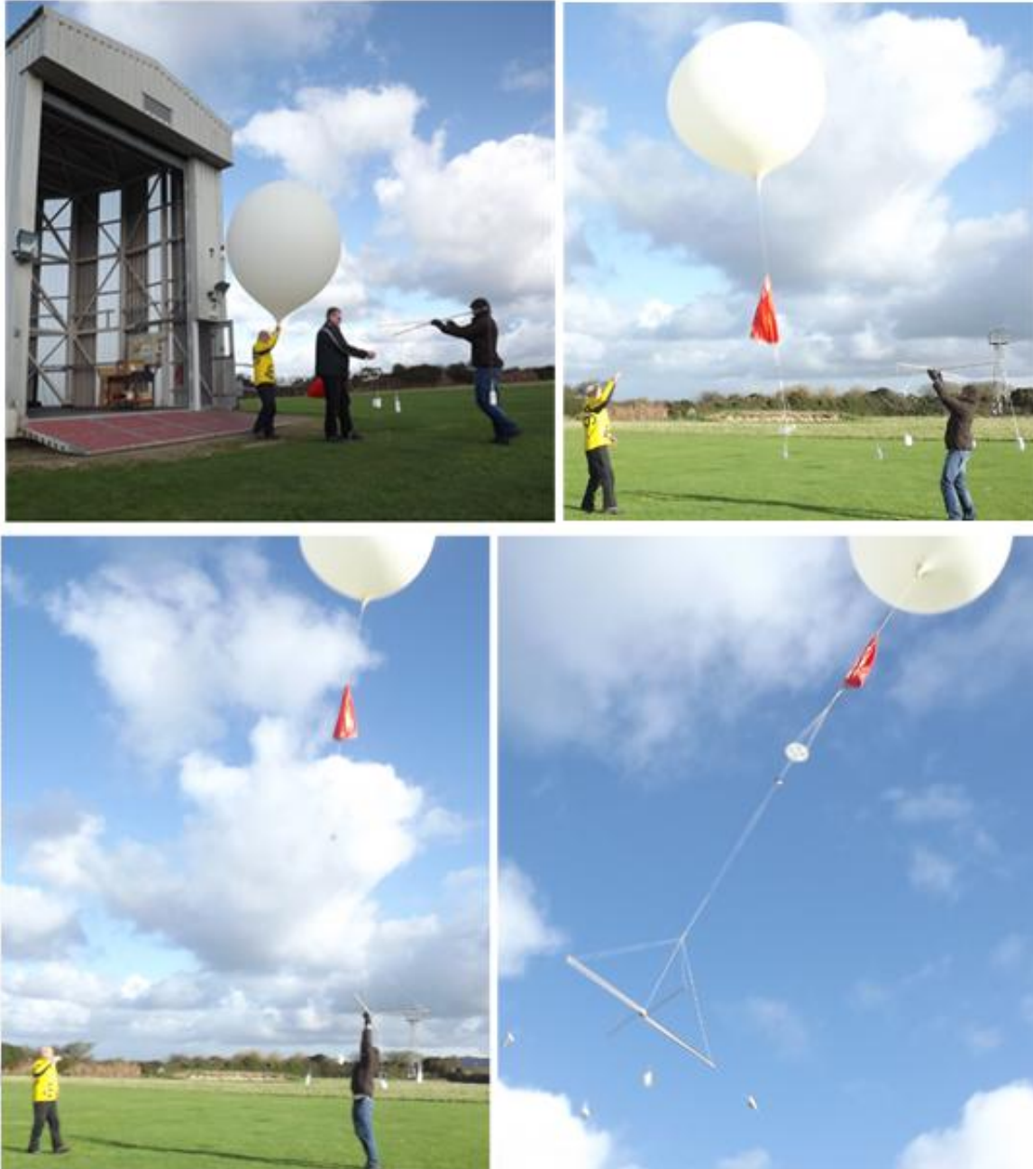
Vaisala staff launching a 4 radiosonde rig used in this report from the rotating balloon shed at the Met Office site in Camborne.
