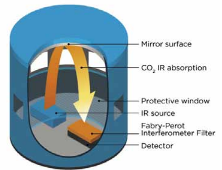
Figure 2. The structure of the Vaisala CARBOCAP CO 2 sensor.
