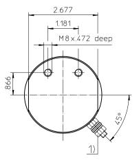
1) Connection for the potential equalization, only for application in the explosive area.
