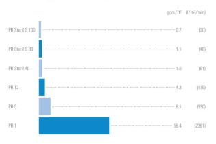
Conditions:  $\Delta$  p = 14.5 psi (100 kPa, 1 bar), Medium: Water at 68 °F (20 °C)
