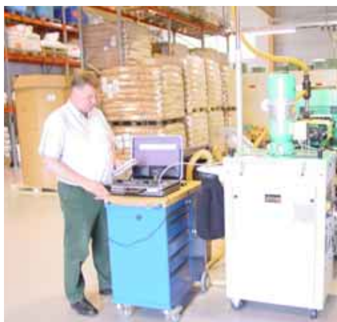
Mechanics Engineer Kari Bergman of Vaisala checks an injection moulding plastic dryer at Plastoco Oy.
