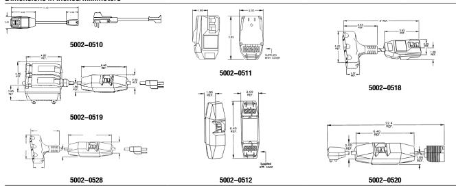
① 2 of the 4 receptacles are T-slotted to allow both 15 and 20 amp tools, with either NEMA 5-15 or 5-20 plugs.
