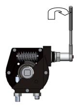
10. The D-Lock is now "engaged" and in the lock out position. Using a 1-1/2" wrench and the 3/4" socket wrench tighten down the lock nut against the lock washer so that the lock washer is completely compressed and flat. (Caution: Do not over tighten.) This process ensures that all of the rotational tolerance stacks in the actuator, D-Lock, and valve have been collected. At this point the valve is torque seated and locked into position.
