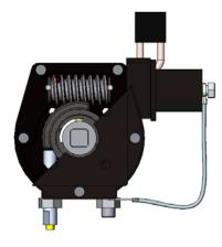
7. When the valve and actuator have been moved to the desired lockout position, full clockwise in this case, the D-Lock is ready to lock out the unit in the lock out position. In this position the valve will not move even if the actuator receives a signal to energize.
