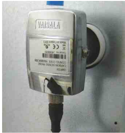
Figure 6. GMP231 probes installed for the incubator test. Outside view (left), inside view (right).
