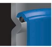
Unique, internal body-to-basket O-ring seal prevents bypass and is easy to maintain
