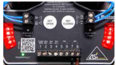
Touch sensors and LED indicators make set up fast and easy.
