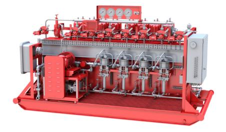
As a crucial component of well control, Cameron land closing units are built to high quality standards and meet API 16D requirements. The land closing units use precharged nitrogen bladder accumulator bottles, hydraulic fluid, and electric- and air-based pumps to generate pressure to operate multiple functions on a BOP stack. Remote panels are offered in electric PLC touch screen, electric PLC push button, or pneumatic air-based remote options.
