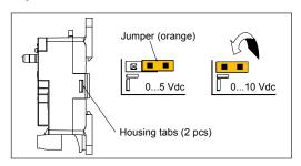
Figure 6 Voltage Output Jumper
