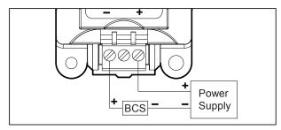
Figure 3 Current Output Wiring
