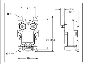
Figure 1 Dimensions (in mm)
