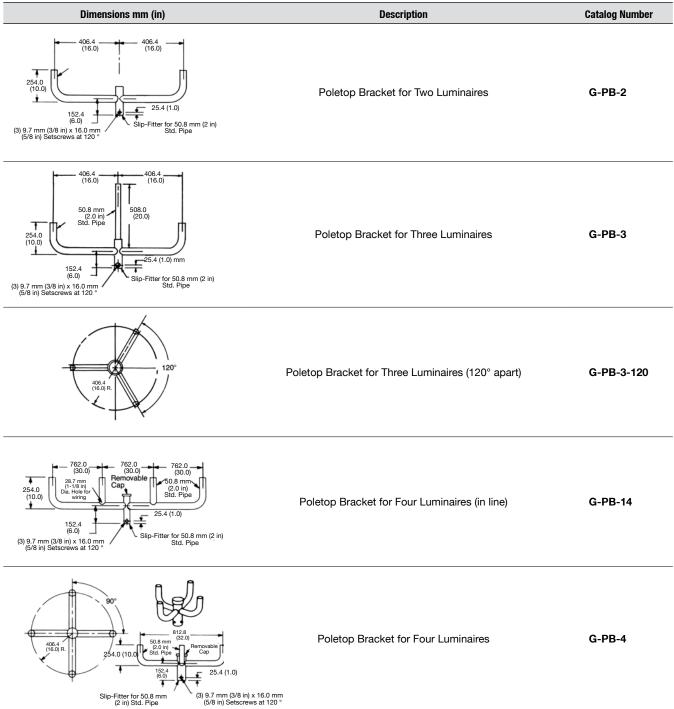
Single or Multiple Installation on Wall, Wood or Metal Poles
