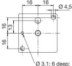
Option for positioning pin ø 3 (ensure correct location for installation)
